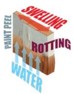
Shrinking and swelling occur from changes in relative humidity in the atmosphere. Water wicks up through wood fibers resulting in paint peeling, rot and mold. Traditional door frames begin to rot within 3-6 months of field installation.
