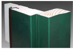
FrameSaver wood frame and brickmold with fingerjointed composite bottom prevents water absorption and carries a Lifetime Limited Warranty when used with PVC vinyl coated aluminum frame cladding outside. Also available with smooth cladding.
